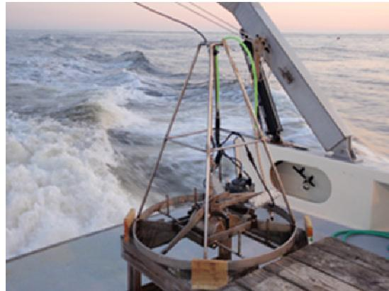
The scientists' grab sampler on the deck of a research vessel
